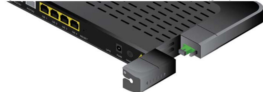
Figure 11: zNID-GPON-24xxA1 models use SC/APC connector (green)
