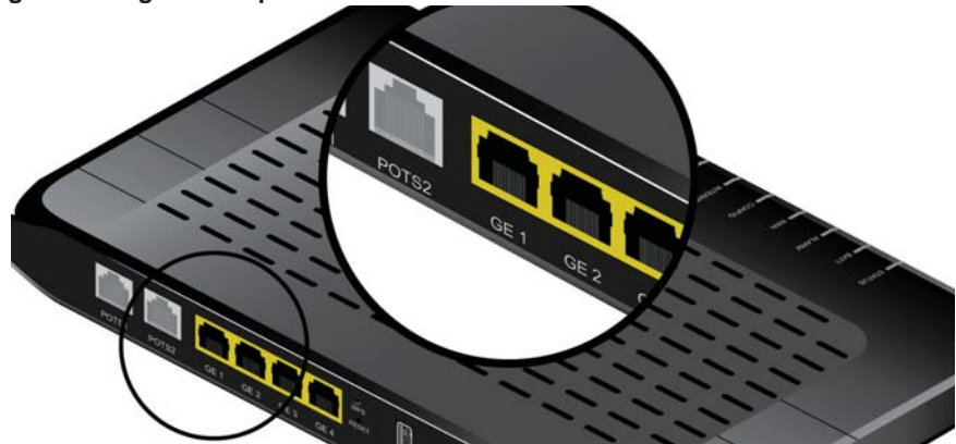
Figure 7: Log into GE port 1 to reach the Web UI or CLI on the zNID
