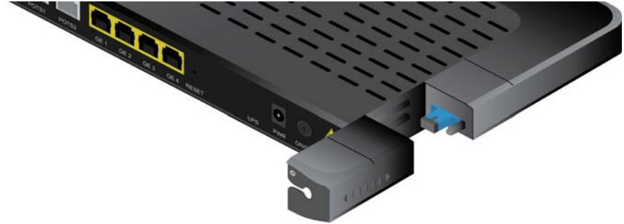
Figure 12: zNID-GE-24xxA1 model uses SC/UPC connector (blue)
