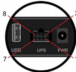
Figure 19: Pin out layout for the UPS connector
