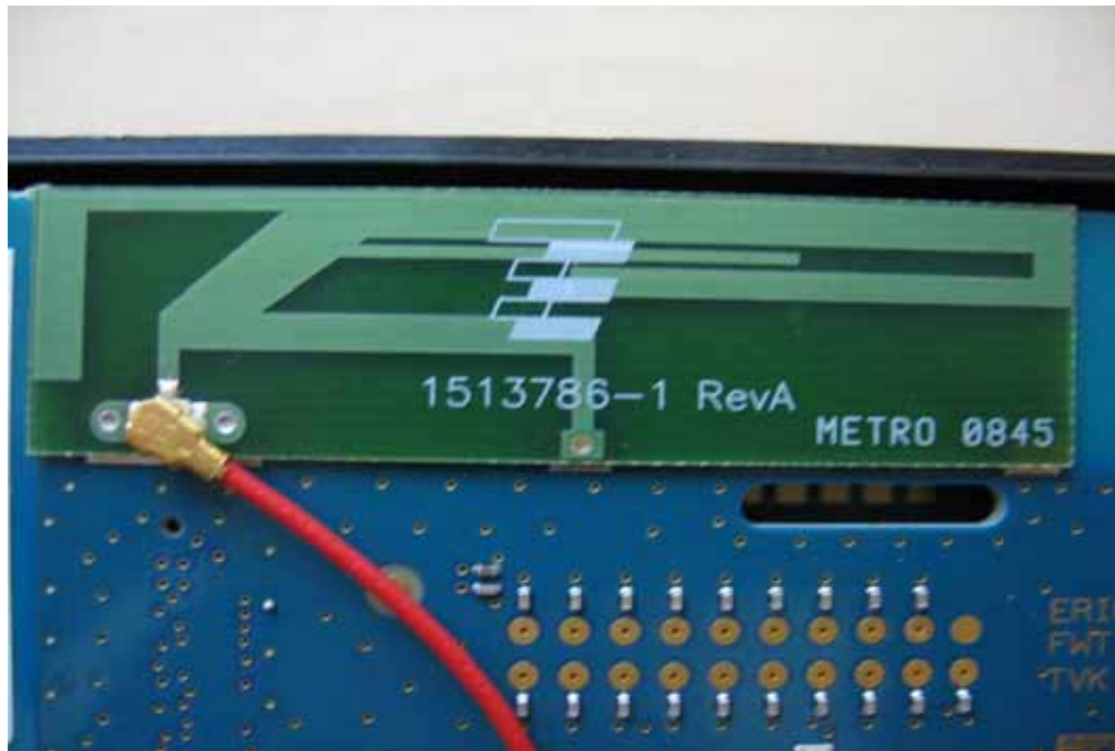
Photo 15: GSM / UMTS antenna
