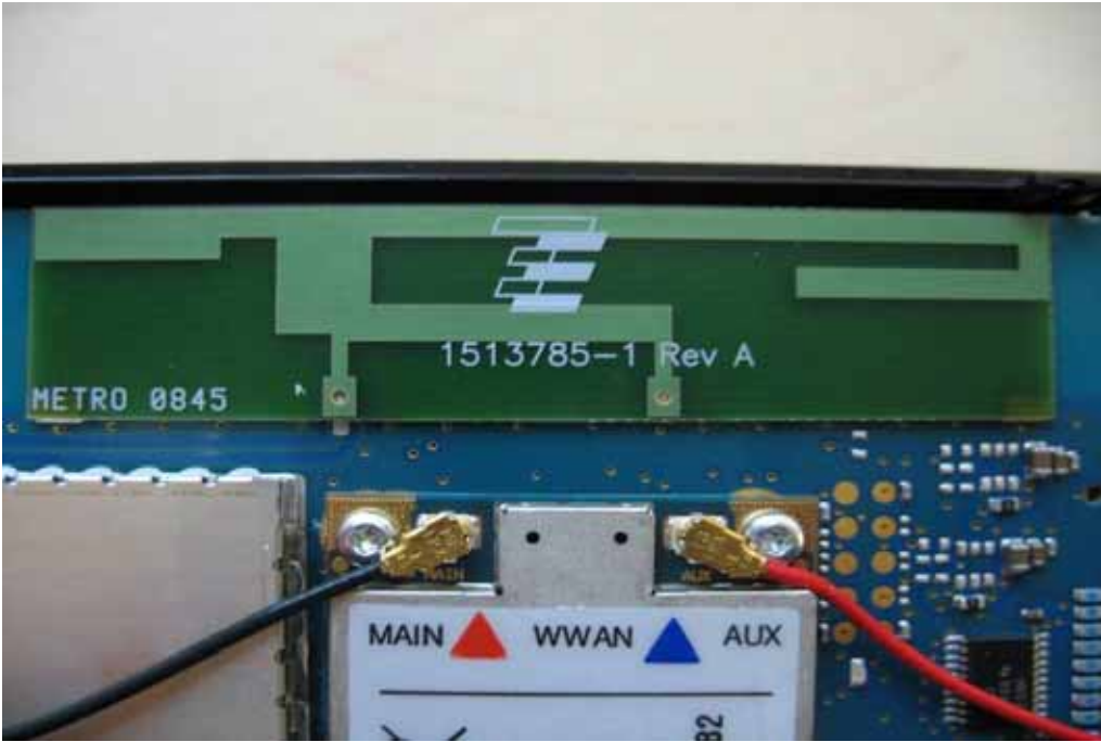
Photo 14: GSM / UMTS antenna
