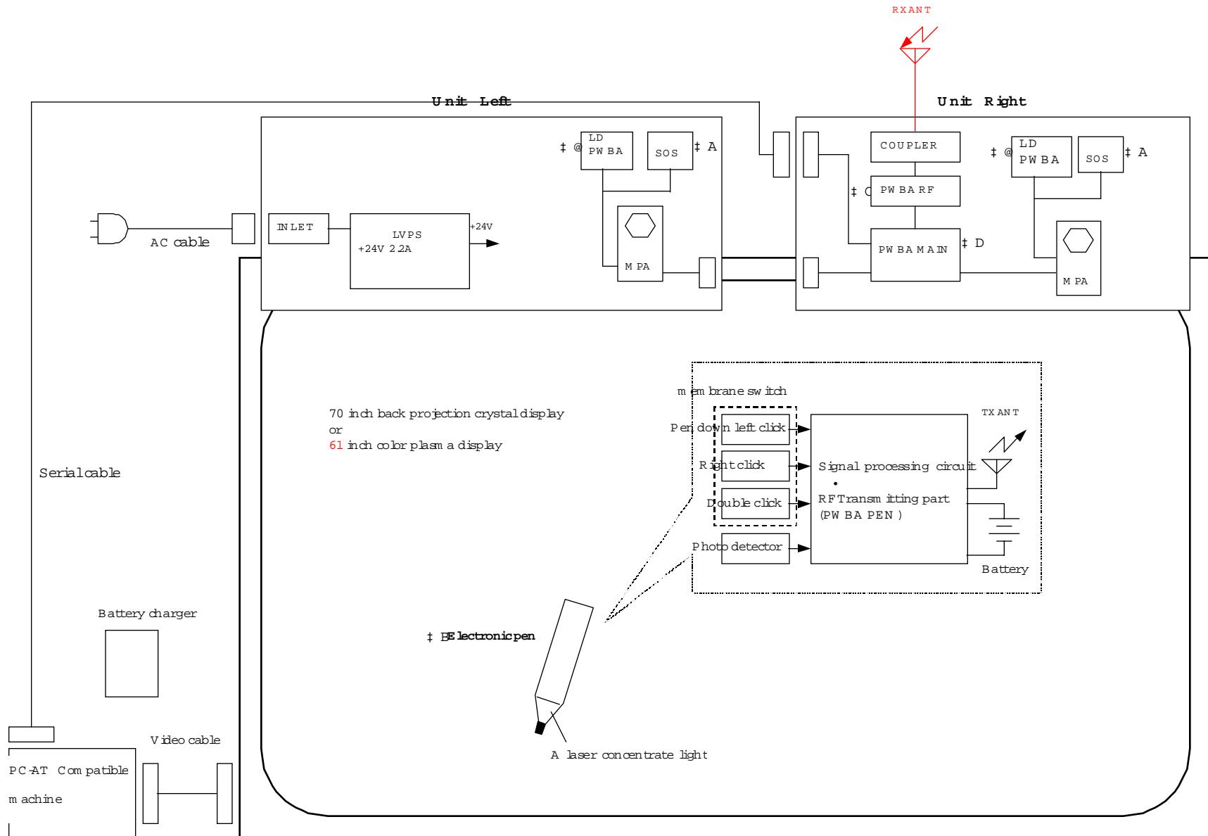
This device detects a position(X,Y) of the electronic pen using two laser scanner units.
