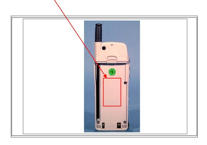
According to the requirement section 2.925 an 2.926, the sample label shown below shall be permanently affixed at a conspicuous location on the device supplied to the user and be readily visible to the purchaser at the time purchase.
