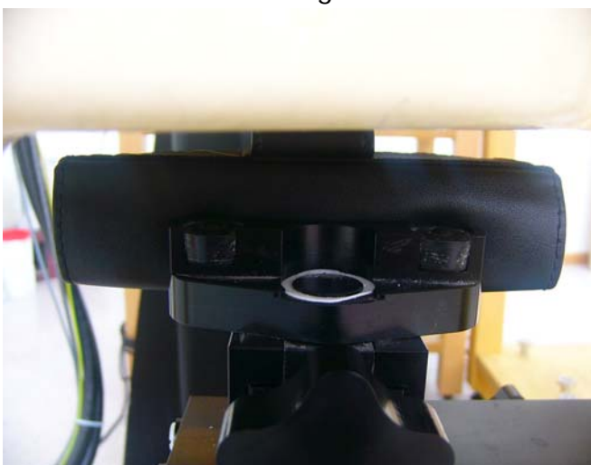
Fig.7 Body worn- EUT front to flat phantom (testing in GPRS Mode)
