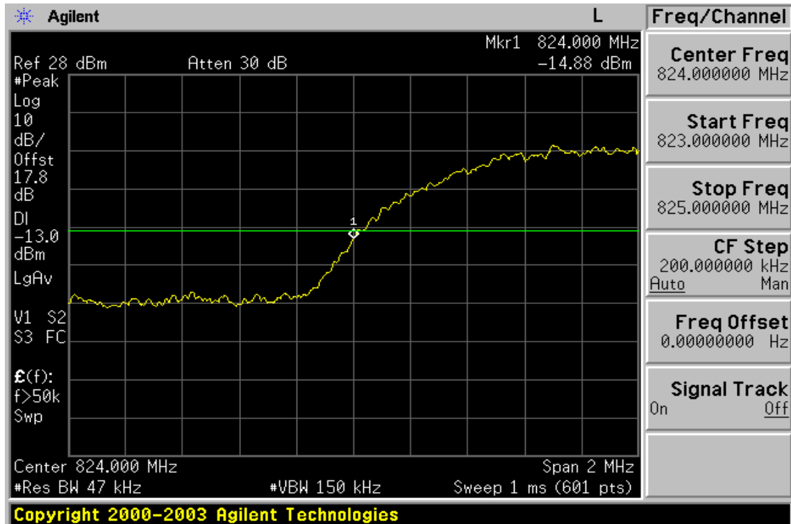
Figure 8-17: Bad edge emission at antenna terminals – WCDMA V Channel Lowest
