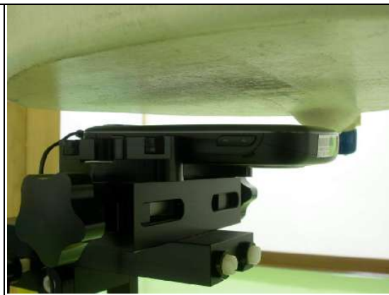
The front of the EUT to the flat phantom distance 15mm.
