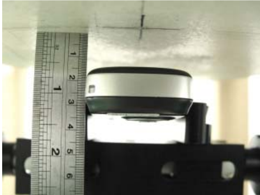
Fig. 9.7 Keypad Up with 1.5cm Gap
