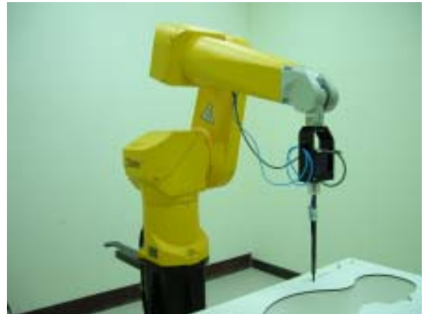
Fig. 5.2 Probe setup on robot
