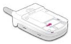
Note: To remove the card, slide it to the left as shown in the diagram below.
