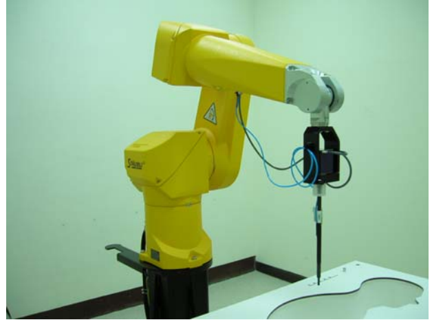
Fig. 5.2 Probe setup on robot
