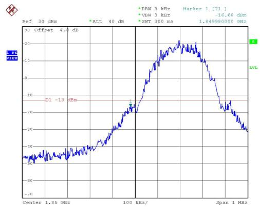
Name of Test: Emission Masks (Occupied Bandwidth) State 2:High Power
