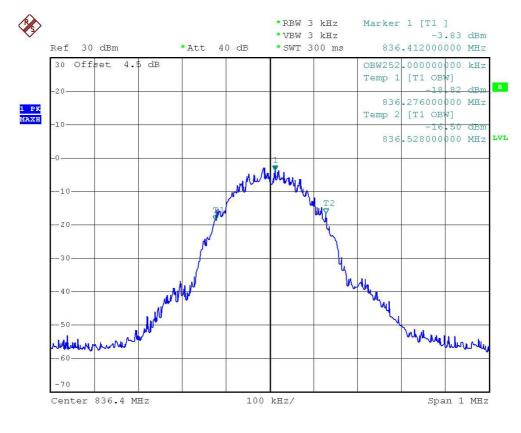
Name of Test: Emission Masks (Occupied Bandwidth) State 1:Low Power
