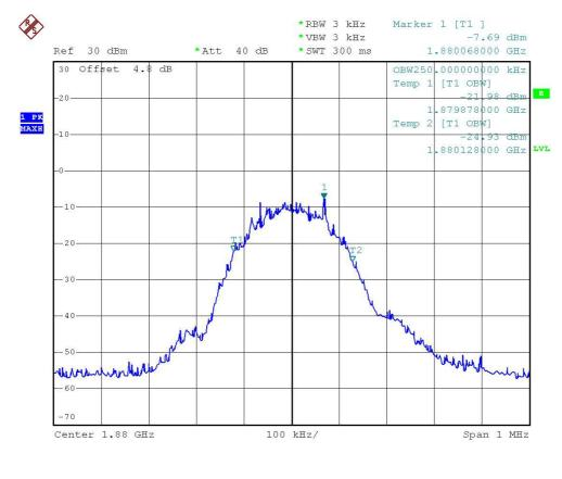
Name of Test: Emission Masks (Occupied Bandwidth) State 1:Low Power
