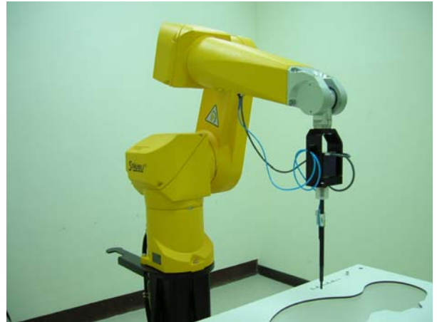
Fig. 5.2 Probe setup on robot
