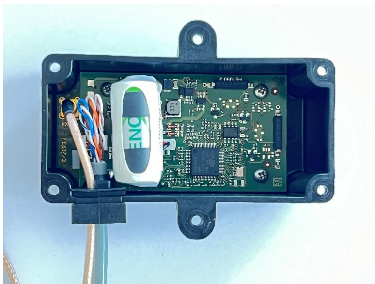
Fig. 2: Internal view of Stationary Wireless Unit FSAS-C (PCB, FE637/3 behind Encoder PCB, FE1090/2) and with plugged-in antenna coaxial connector
