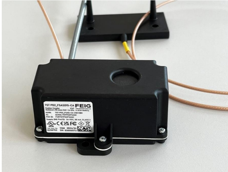
Fig. 1: External view of Stationary Wireless Unit FSAS-C fitted into Encoder Housing TST PD2_FSAS-C and antenna
