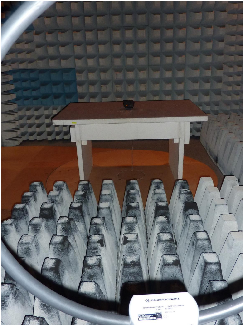
160532_103.jpg: MWD BPC-HU, test setup fully anechoic chamber <1 GHz
