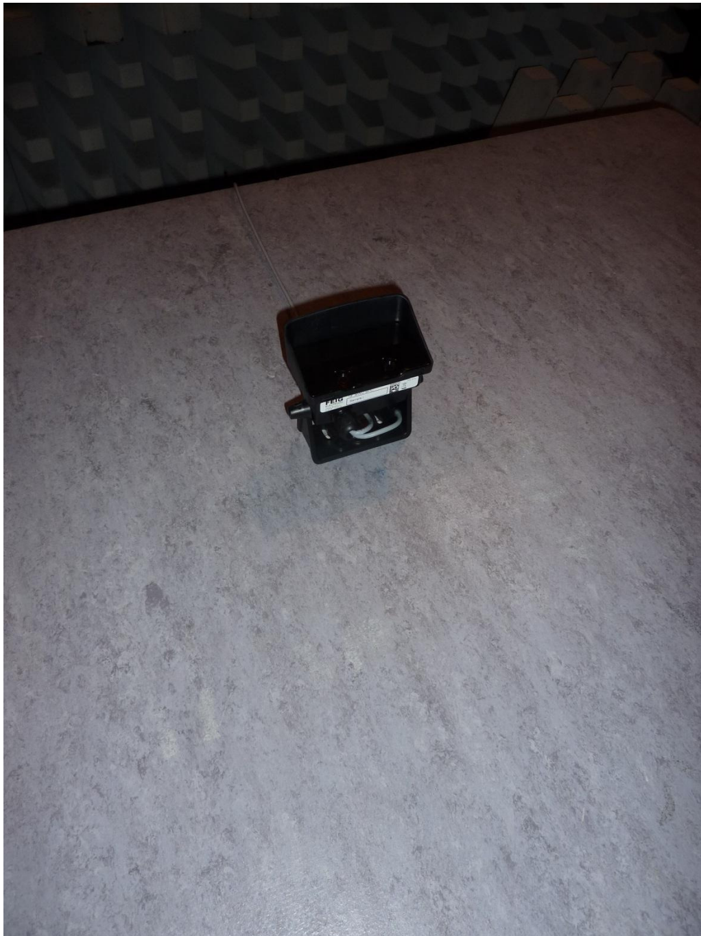
160532_101.jpg: MWD BPC-HU, test setup fully anechoic chamber (pos. 2)
