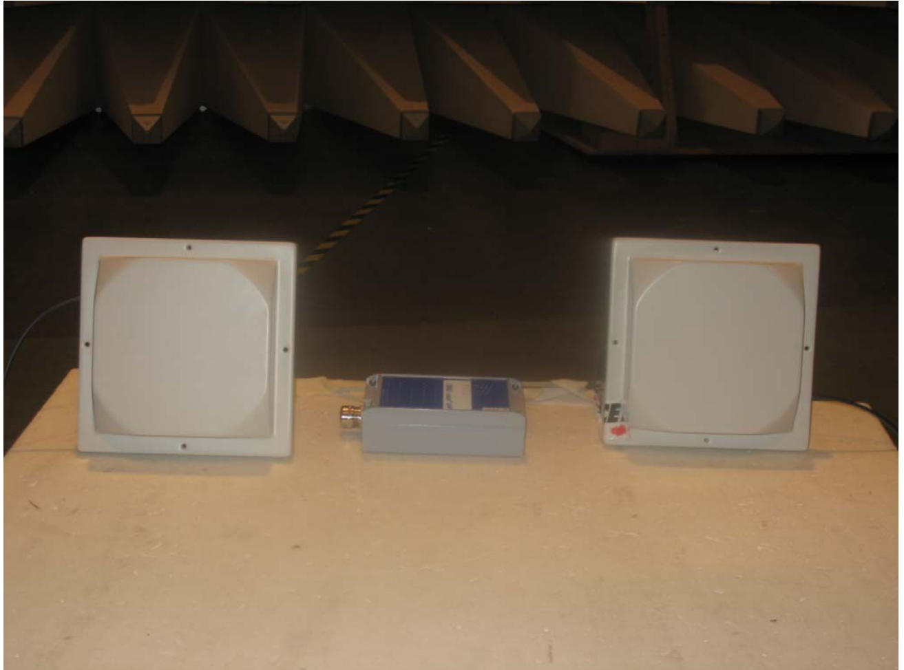
Photo 1: Radiated Emissions with housing
