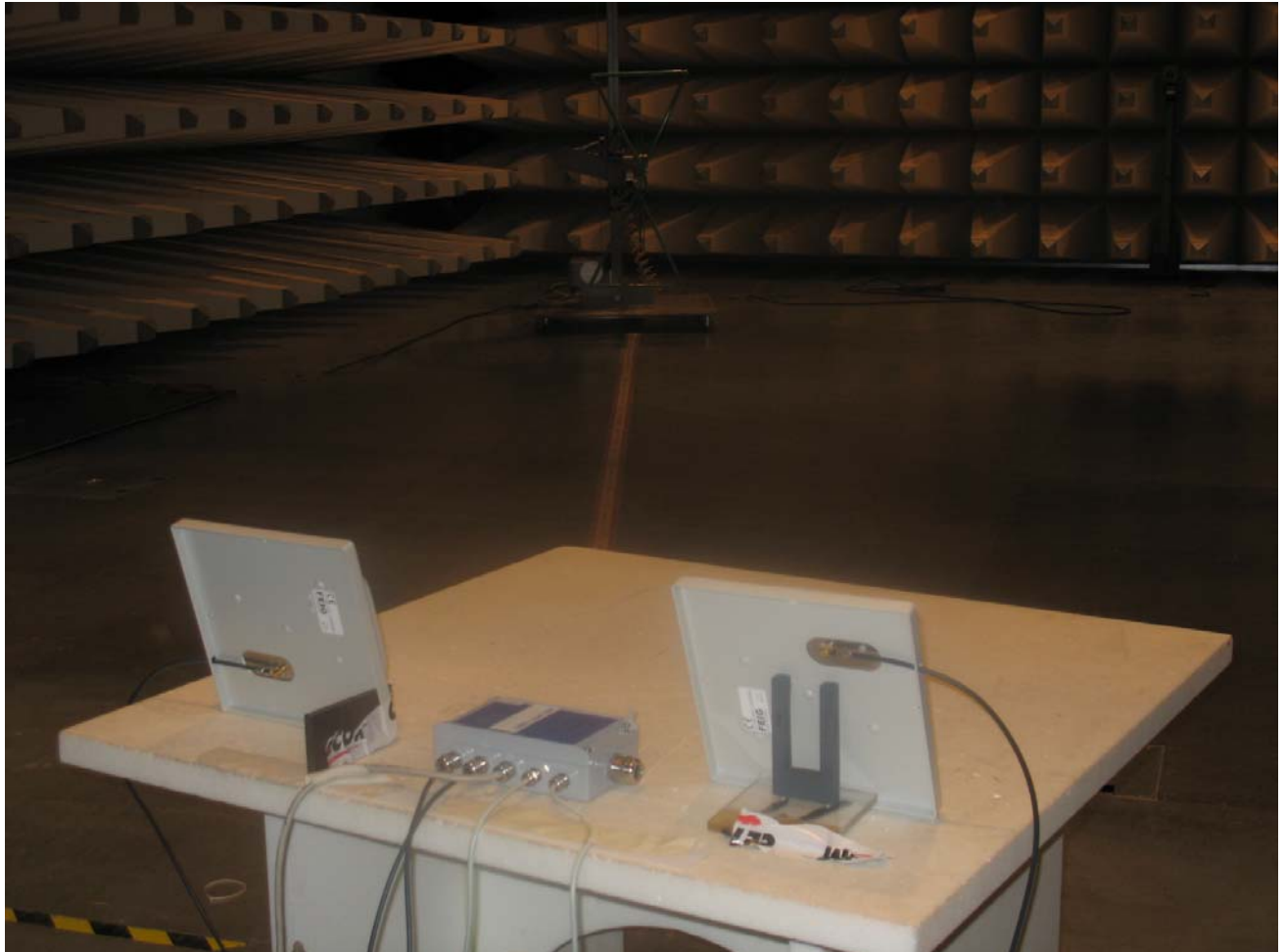
Photo 2: Radiated Emissions with housing
