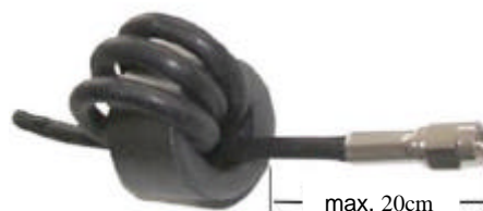
Fig. 3-6: Antenna cable with EMC ferrite ring core
