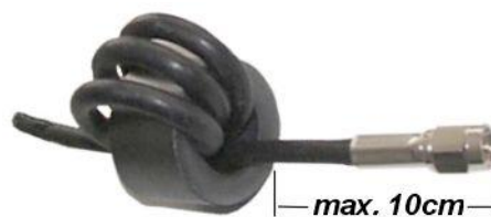
Figure 3: Assembly of the torrid core at the coaxial cable
