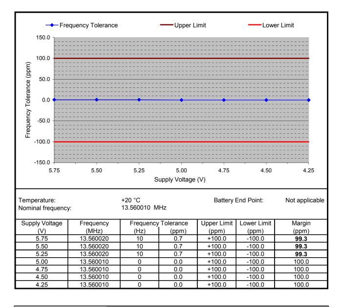
Test Result: Test passed
