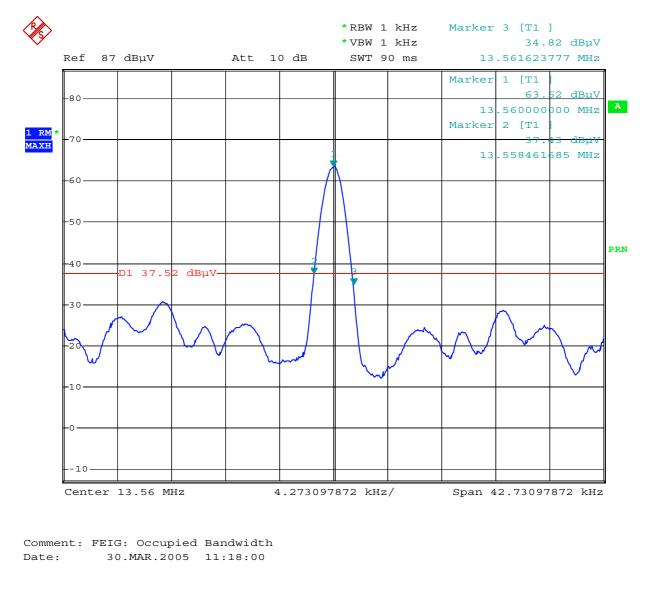
Occupied Bandwidth (-26 dB): 3.16 kHz
