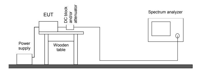
Test instruments used for conducted measurements:
