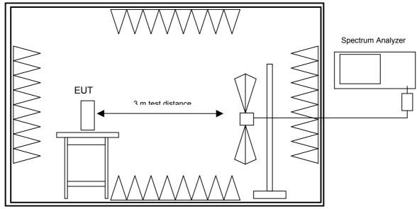
Fully anechoic chamber
