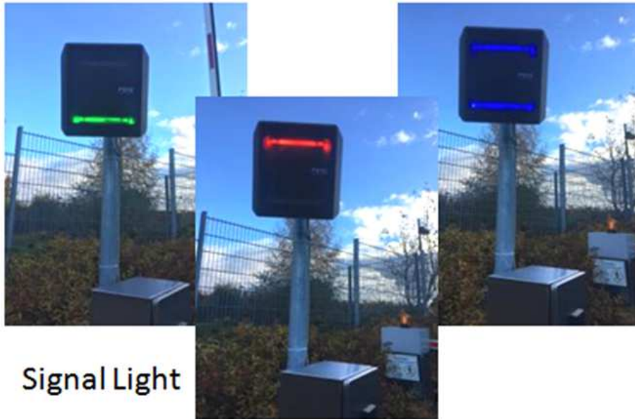
Image 1: Reader mounted on pole with signalling LEDs active
