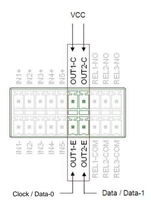
Fig. 11: Data-Clock Interface on connector X5
