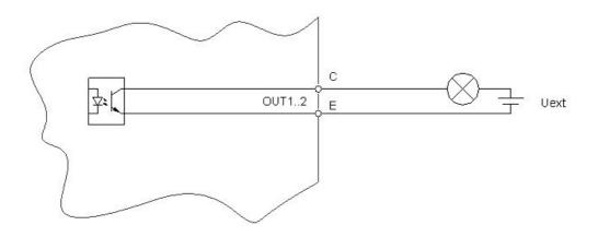
Fig. 16: Internal and external wiring of the optocoupler-outputs OUT1-2
