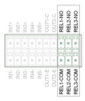
Fig. 17: Relay output pin-outs REL1-3
