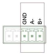
Fig. 10: RS485 interface pin-outs on X6 (RS485-Interface)
