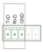
Fig. 8: RS232 interface pin-outs on X6
