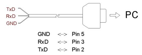
Fig. 9: Wiring example for connecting the RS232 interface X6
