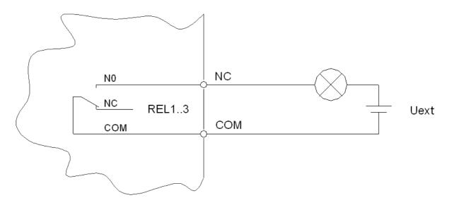
Fig. 18: Internal and external wiring of the relay output
