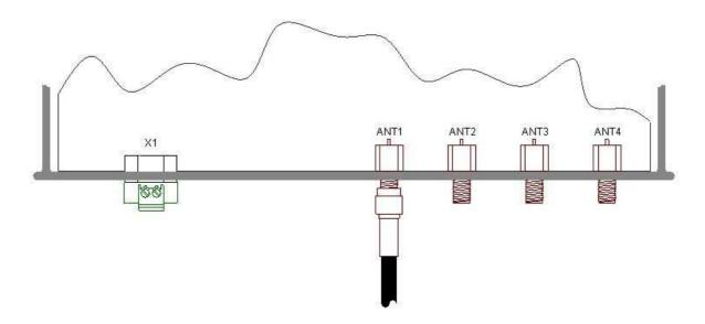
Fig. 3: External antenna connection ANT1-4 and X1 for the power supply
