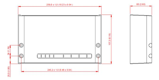
Fig. 1: Installation Drawing
