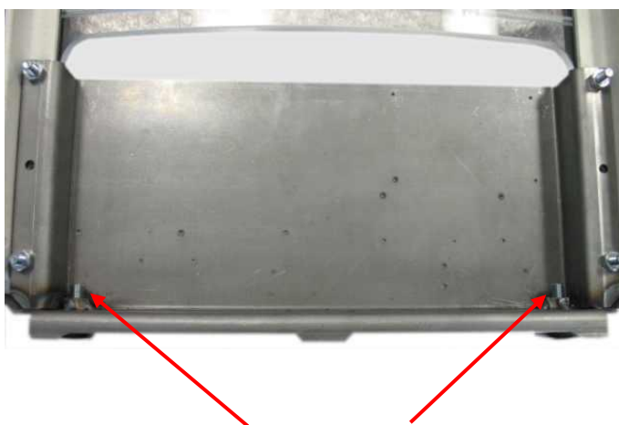
Adjusting screws (hexagon socket width AF 4)
