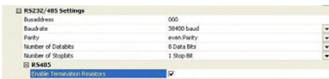
Fig. 25: Jumper settings RS485 Interface
