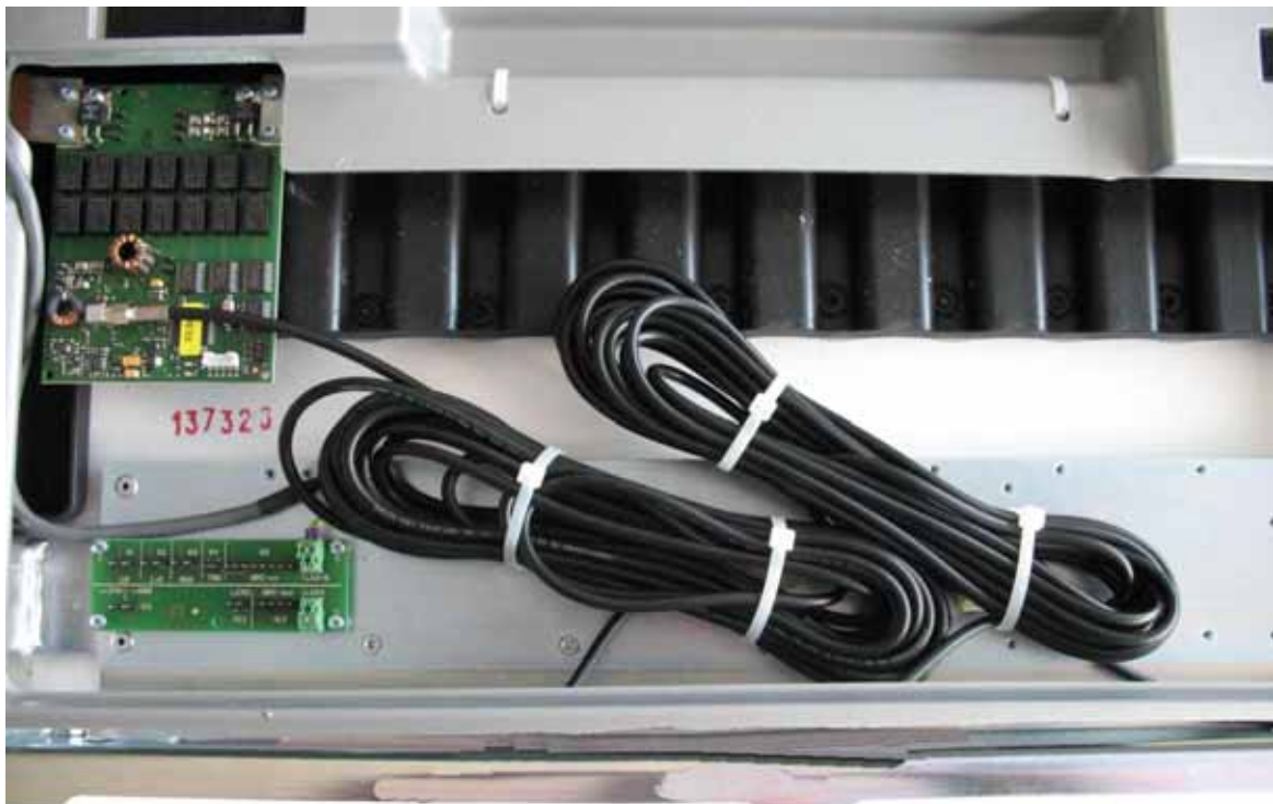
Fig. 14: Tie together the cables in an antenna Type B
