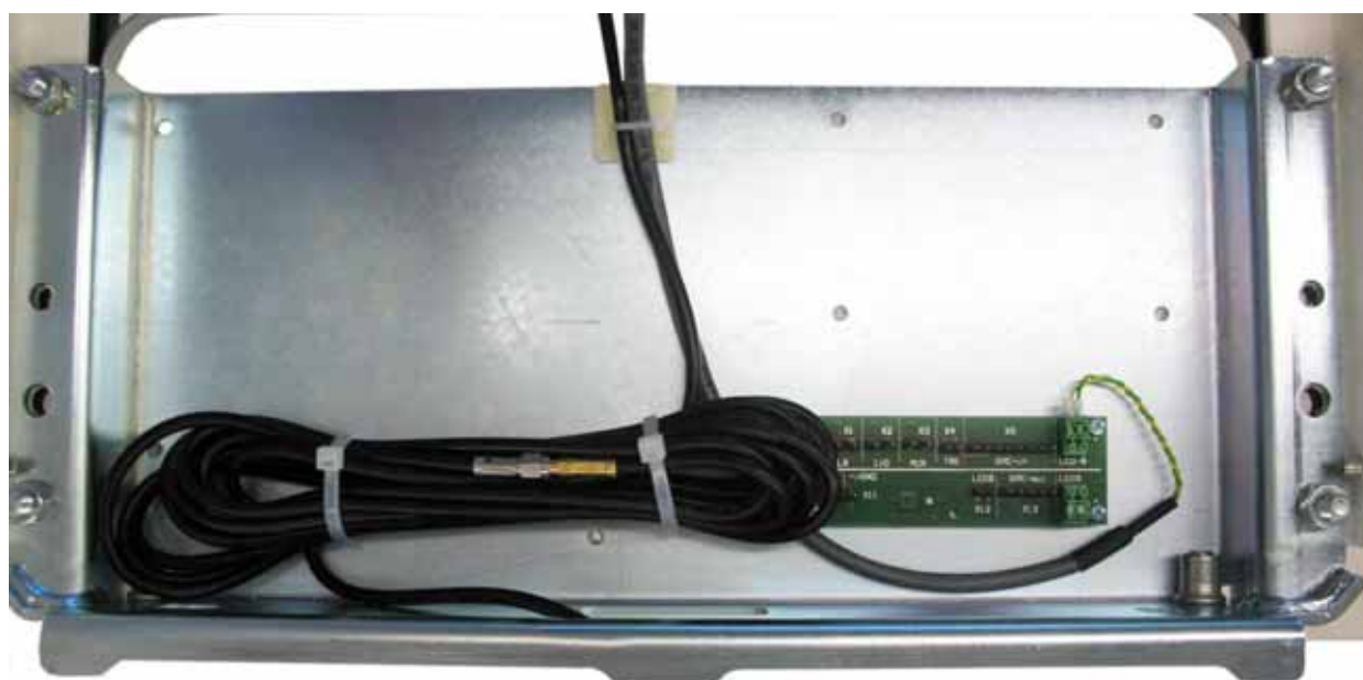
Fig. 14: Unused coaxial cables are tied in antenna Type B
