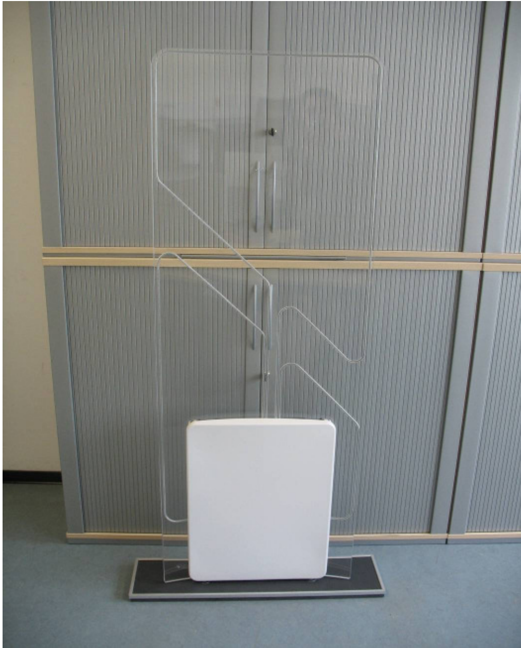
Gate 2 (multiplexer & reader)
