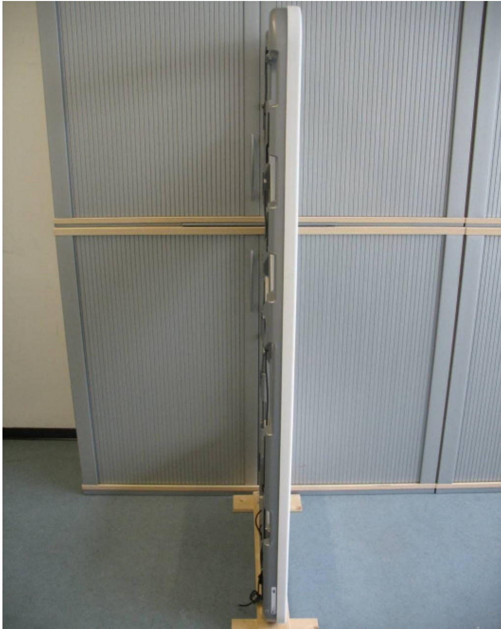
Gate 2 (multiplexer & reader)
