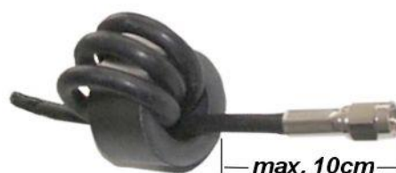
Figure 3: Antenna line with EMC ring cores
