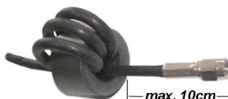
Figure 5: Antenna line with EMC ring cores
