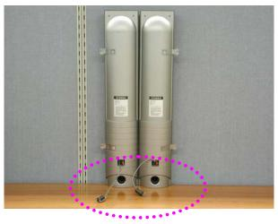
6. The wires which connected DVI ground pin and PCB ground, will be modified with PCB pattern artwork
