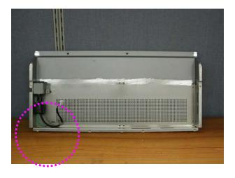
3. Attach a copper foil between main frame and EMI filter shield
