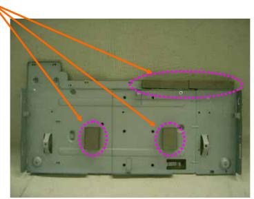
6. Attach a gasket on the main board case.
