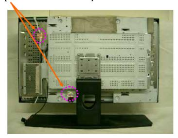
2. Apply a ferrite core to the interface Cable of MMB Board.
