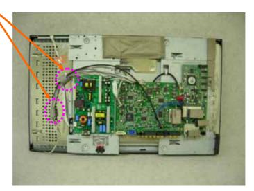
3. Attach fabrictape and a gasket on the frame.
