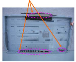
5. Attach a gasket on the LCD Panel Rear cover
