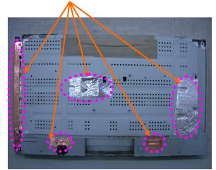
2. Attach fabrictape on the Rear frame.
