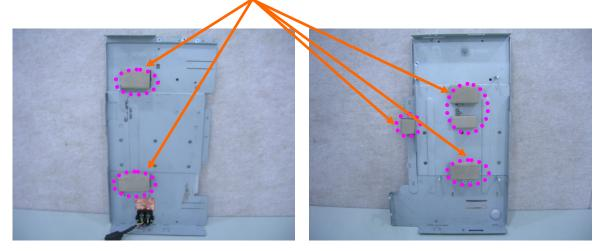
6. Attach aluminum tape on the LCD Panel Rear cover
