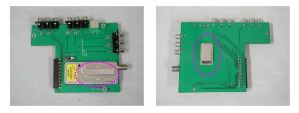
5. Attach a gasket on the main board.
