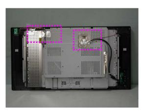
2. Attach a gasket on the main frame cover inside.
