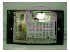
2. Attach a gasket on the main board.
