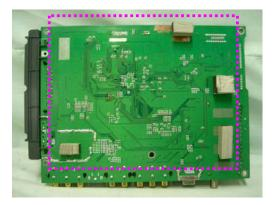
3. Attach aluminum foil on the mainframe cover for OSD and audio signal cable fixed.
