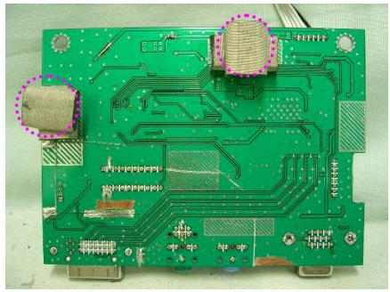
4. Apply a strip of aluminum tape on the conductive strip to the frame.
