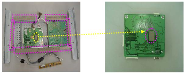
3. Attach a gasket on the Audio PCB to contact a stand
