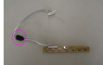
6. The wires which connected MCU and video decoder chip, will be modified with PCB pattern artwork
