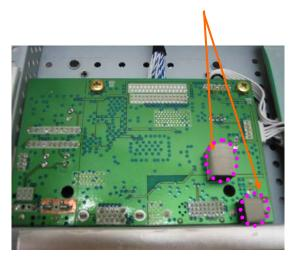
3. Attach aluminum tape on the Rear frame.
