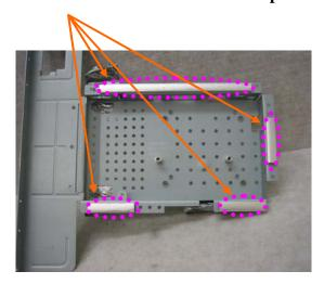
2. Attach a gasket on the main board to contact the main frame
