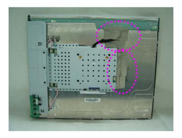
2. Attach a gasket on the main frame to contact the lcd panel
