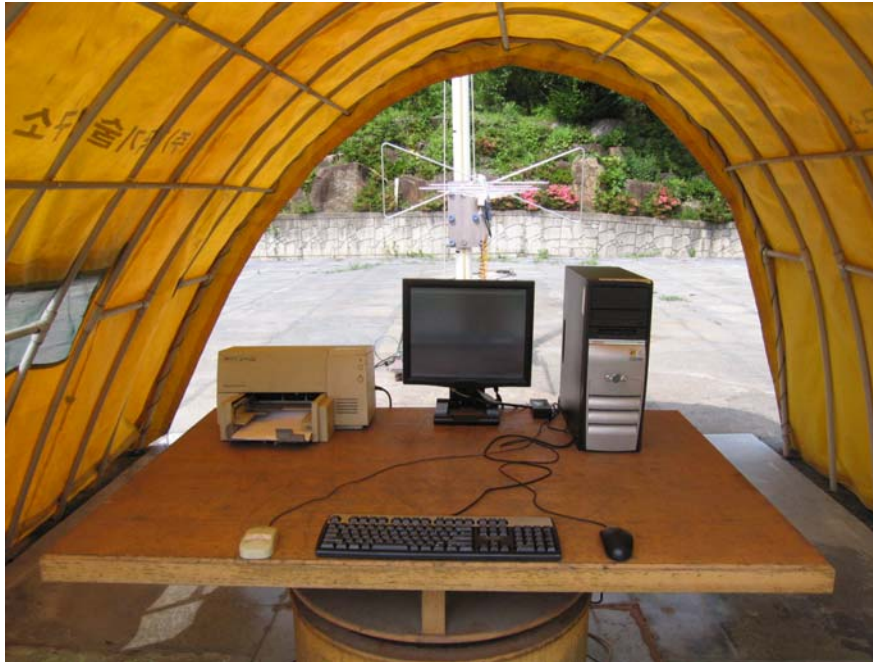
Photograph 1 : Setup for radiated Emissions
