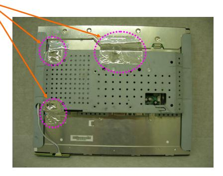
2. Attach a gasket on the main frame to contact the lcd panel.
