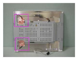
4. Apply a ferrite Core to the OSD board signal cable
