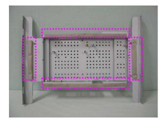
2. Attach a copper foil between Main Frame and LCD panel
