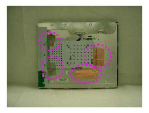
2. Attach a gasket on the main frame and main board to contact the lcd panel
