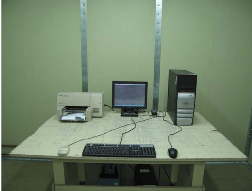
Photograph 2 : Setup for Conducted Emissions
