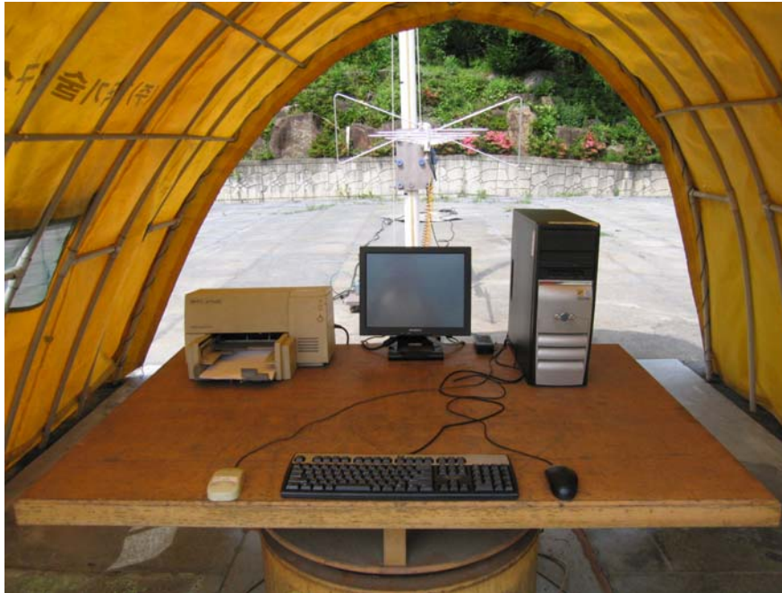
Photograph 1 : Setup for radiated Emissions
