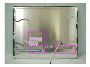
2. Attach aluminum foil between Main Frame and LCD panel
