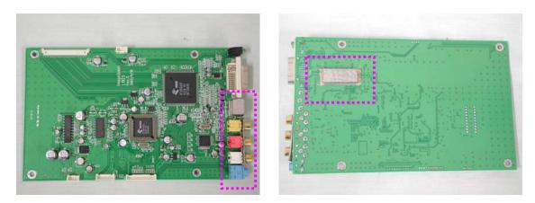
**3.** Attach a gasket on the LCD panel
