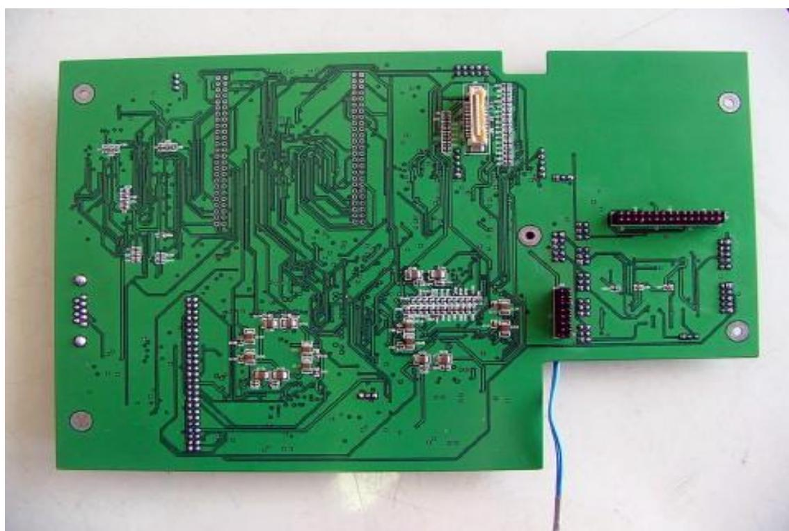
**CONSTRUCTED PHOTOS of EUT****7. Component View of HDSL Card**
