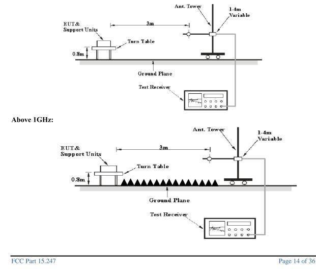
The radiated emission tests were performed in the 3 meters test site, using the setup accordance with the ANSI C63.4-2009. The specification used was the FCC 15.209, and FCC 15.247 limits.
