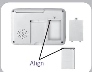
For added portability, the rechargeable battery for your monitor will provide approximately 5 hours of video usage and 10 hours of audio only usage.
