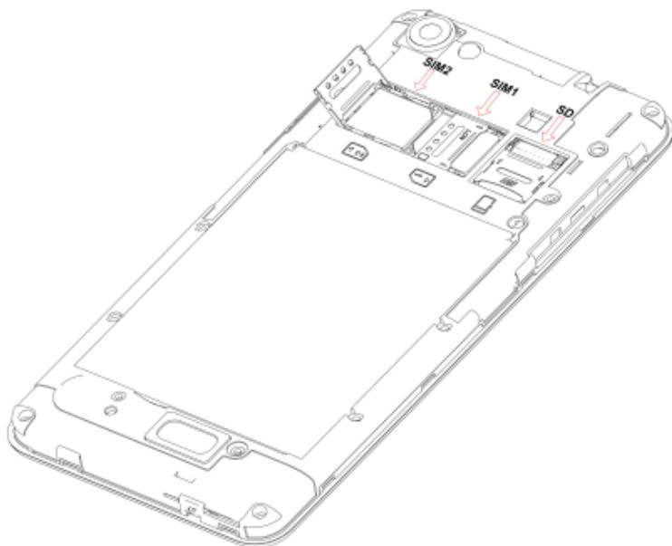
SIM Slot 1: Micro SIM card slot
